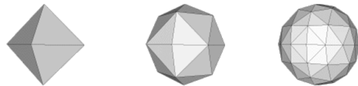
Figure 1. Decomposition of the Earth's surface for triangular meshes with resolutions of zero, one, and two.
