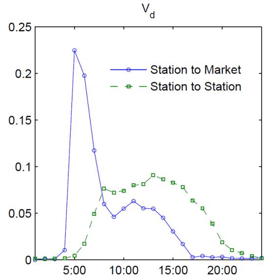
**Figure 6.  $V_d$  of OD flow from Station to Market and OD flow from Station to Station. Note that commute flow(Station to Market) aggregate in early morning while transfer flow(Station to Station) is flat distributed in day-time.**
